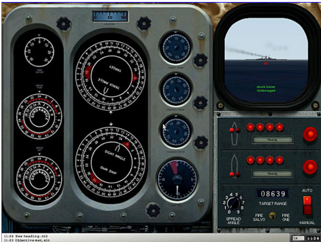
Figure 7 - An ideal shot as seen from the torpedo director station in the torpedo training scenario. The torpedoes have a crossing angle of near 90^\circ , they are at their fastest speed setting and the run time is less than one minute. Due to the high torpedo speed (45 knots) and the low speed of the target vessel (10 knots), the sight angle is very small, about 15^\circ here.
