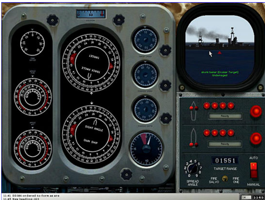
Figure 7 - An ideal shot as seen from the torpedo director station in the torpedo training scenario. The torpedoes have a crossing angle of near 90^\circ , they are at their fastest speed setting and the run time is less than one minute. Due to the high torpedo speed (45 knots) and the low speed of the target vessel (10 knots), the sight angle is very small, about 15^\circ here.
